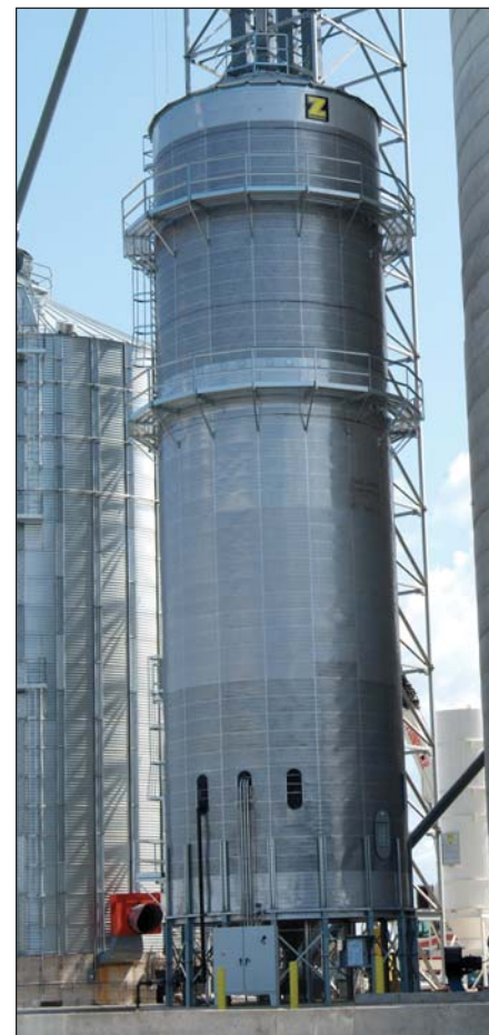
LP-gas Zimmerman tower dryer has the capacity to dry 5,000 bph of grain at five points of moisture removal.
