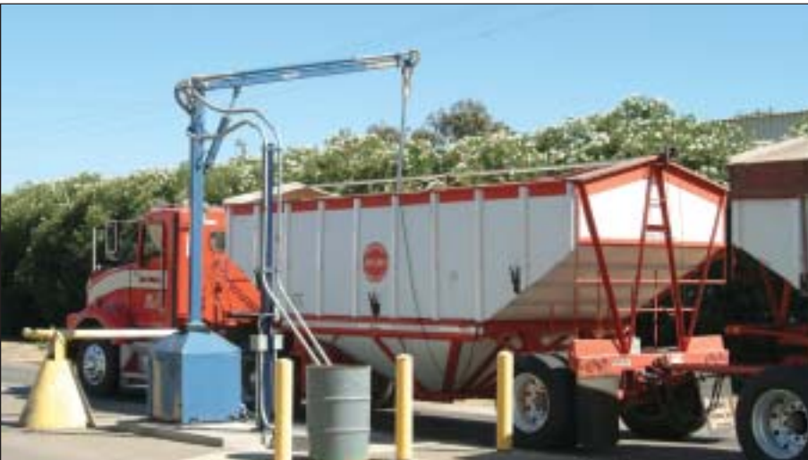
An incoming truckload of grain at the Road 102 elevator is sampled with a CR Mfg. Shuttle grain probe prior to weighing.
