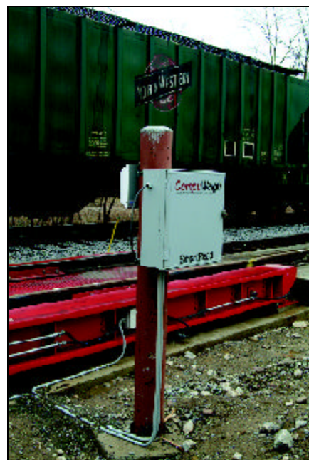
CompuWeigh SmartRead station transmits railcar identification and capacity data from railcars parked on the rack scale to the GMS via radio.
