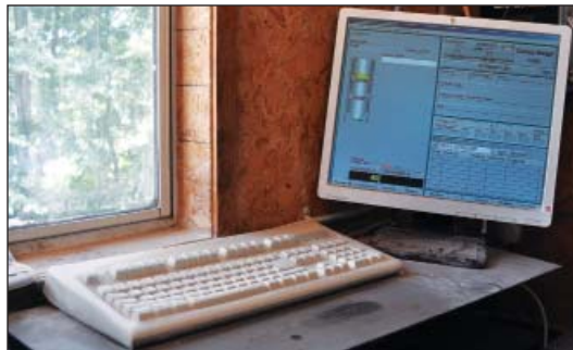
GMS 4000 workstation inside the rail loadout shed, which receives input from CompuWeigh's SmartRead system that gathers data from railcar-mounted RF tags and accesses a North American database that includes capacity information for every railcar on the continent.
