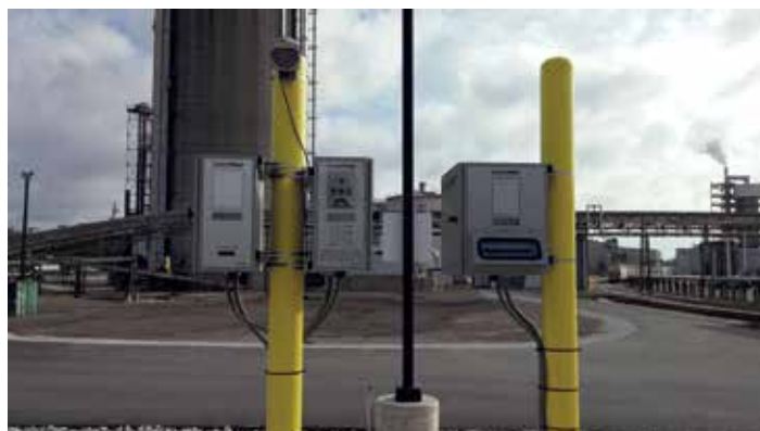
SmartCom allows drivers to enter Load-order Numbers. SmartTalk from CompuWeigh provides clear audio and video communication between drivers and staff
