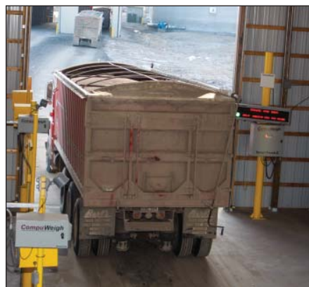
Truck exits inbound probe station and is directed by the SmartTruck system to one of three receiving pits.
