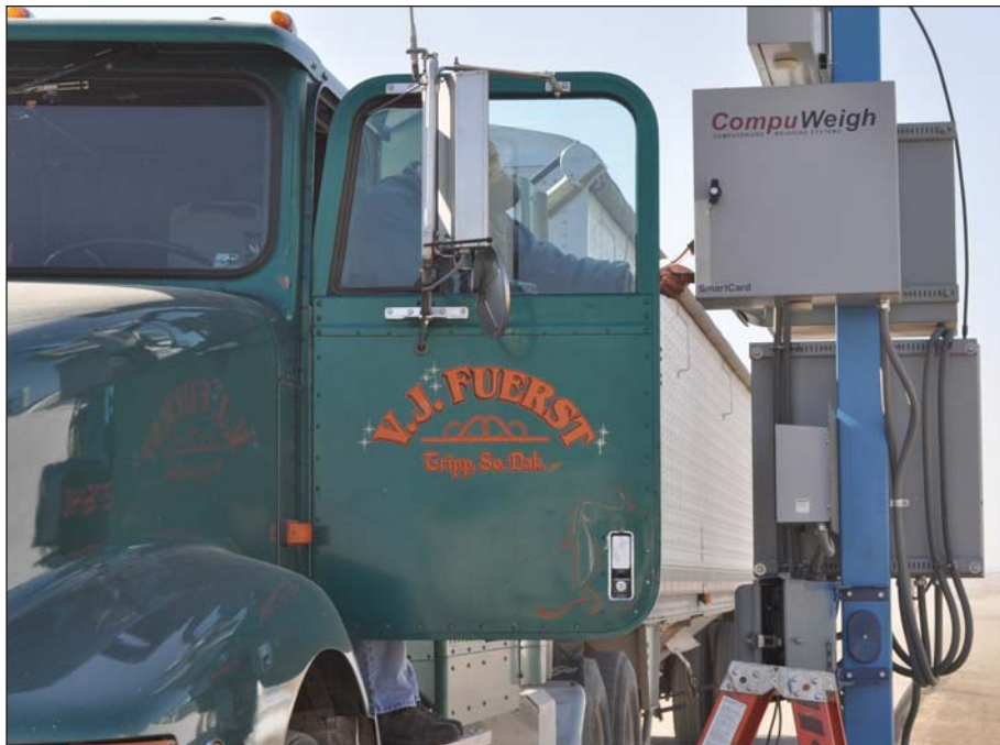
Driver picks up a scale ticket from a SmartCard printer adjacent to the outbound scale prior to departing the Dakota Plains facility.
