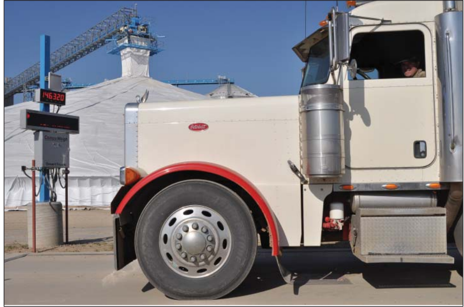
Trucker is weighed on an inbound scale and awaits assignment to a receiving pit through a CompuWeigh SmartChoice module at Dakota Plains Ag Center near Parkston, SD. Photos by Ed Zdrojewski.
