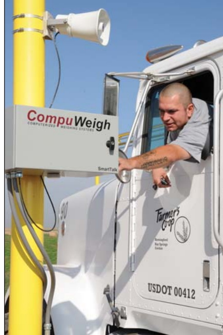
A trucker on the unattended outbound scale has a question and uses the SmartTalk intercom system to call the control room.
