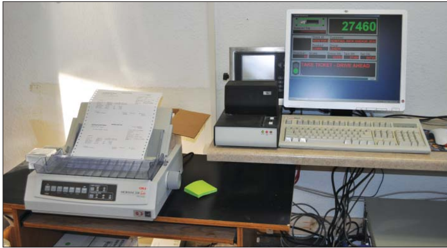
Outbound scale PC in unattended mode processing trucks without human intervention. An "inside copy" of each transaction is printed by the form printer in the office.
