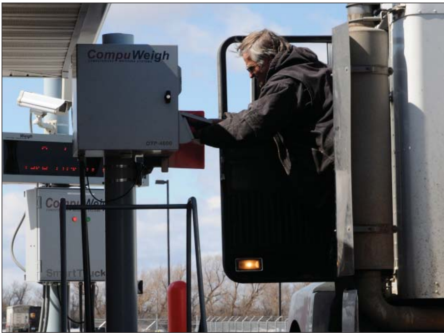
Trucker receives a scale ticket from a printer adjacent to the outbound scale, all part of a CompuWeigh SmartTruck traffic management system at Hankinson Renewable Energy's ethanol plant at Hankinson, ND. Photos by Rob Siverson, Fargo, ND.
