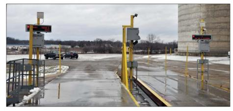
CompuWeigh SmartTruck equipment installed on a truck probe lane (left) and outbound scale (right) at Kokomo Grain in Edinburgh, IN include RF tag readers, SmartView message boards, and video cameras. Photos by Ed Zdrojewski.
