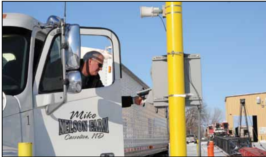
Driver receives a scale ticket from a CompuWeigh OTP-4600 outdoor ticket printer without having to leave his cab.
