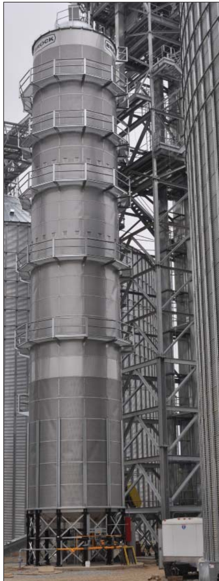
Brock tower dryer is fired by natural gas and rated at 4,700 bph at five points of moisture removal.
