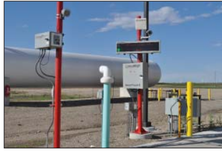
CompuWeigh SmartTruck system guides drivers through the Pillsbury property. In the background, a propane tank supplying a 7,000-bph Zimmerman grain dryer.
