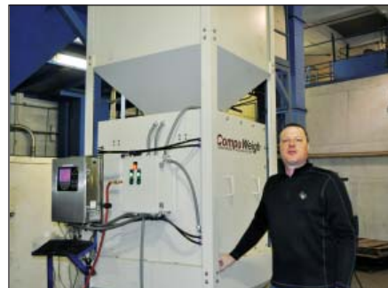
General Manager Nick Shockman with the new CompuWeigh process hopper scale.
