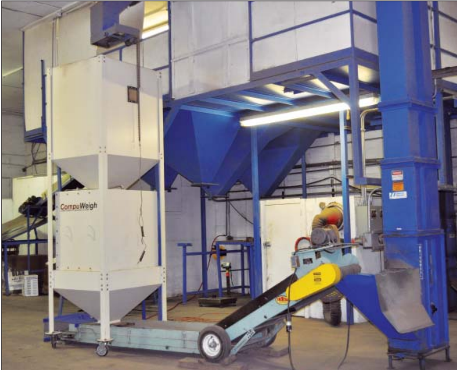
New CompuWeigh process hopper scale is used to generate accurate rates for loading railcars at Larson Grain Co.'s dry edible bean processing plant in Englevale, ND. Photos by Ed Zdrojewski.
