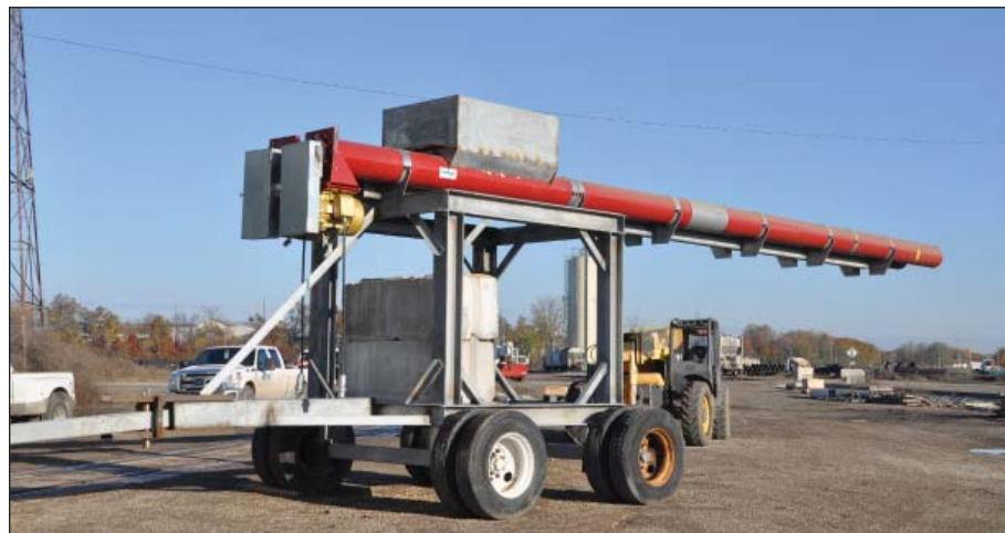
Portable auger system has been loading grain from the facility bulkweigher directly into 40-foot shipping containers.
