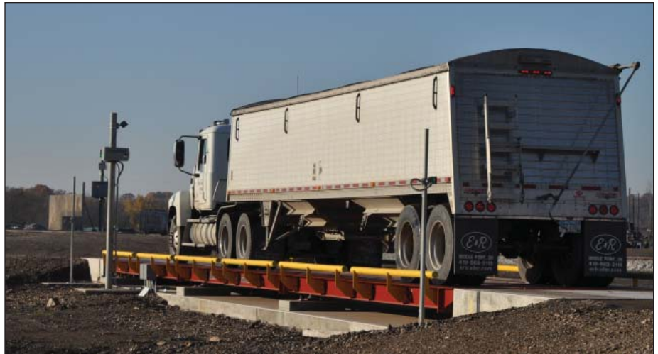
Inbound truck is weighed on a 72-foot Brechbuhler scale while the driver awaits instructions via a CompuWeigh SmartView digital message board. Ground-level photos by Ed Zdrojewski.
