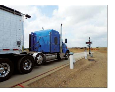
CompuWeigh Corp.'s SmartTruck is a sophisticated but easy-to-use automated truck weighing system that allows users to process more trucks in less time. SmartTruck combines longrange RF cards, outside message boards, electronic photo eyes, video surveillance cameras, noise cancelling intercom systems, electronic signature pads, driver's license readers, and a powerful computer system configured to the needs of the individual facility.
