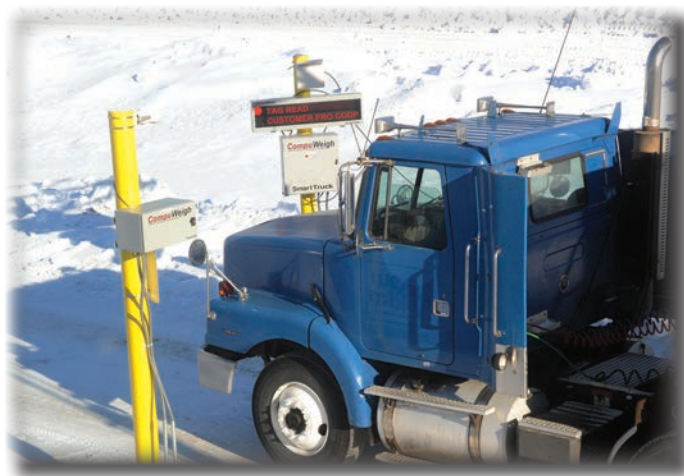
SmartTruck System with automatic RF identification, message board and remote communication system
